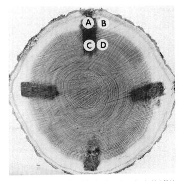
Fig. 1. Compartmentalization of discolored wood associated with drill-bit wounds in red oak after 2 yr. Cross section is 5 cm above the drill wounds. Electrical resistance was measured and wood samples for elemental analysis were taken at positions shown: A, discolored sapwood; B, sapwood; C, discolored heartwood; D, heartwood.
