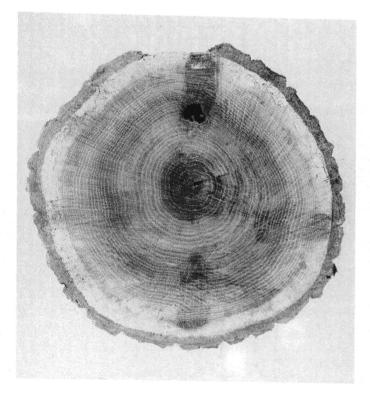
**Fig. 2.** Incomplete compartmentalization of discolored heartwood associated with four drill-bit wounds after 2 yr in red oak that was girdled immediately after wounding. The trees were dead at harvest. Cross section is 5 cm above the drill wounds.
